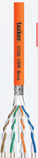
tasker® C722 CPR B2ca C 722 CPR B2ca Section: 4x2x0,25 mm 2 - 7,50 mm - Cat. 6 CPR B2ca Class Sheath: LSZH CPR
