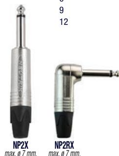
Premade audio cable with jack mono male 6.3 (NP2X) and 90° jack mono male 6.3 (NP2RX). Shielded unipolar cable 1x0,50 mm<sup>2</sup> with carbon screen, available in sizes of 3, 6, 9 or 12 meters. Metal shell connectors impact resistant.
