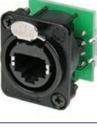
Connettore EtherCON cat.5e femmina, da pannello, con corpo in metallo, contatti dorati e terminali a perforazione d'isolante (IDC).<br>Female EtherCON cat.5e panel connector with black metal body, gold contacts and insulation displacement termination (IDC).                                                                                                                                        |
